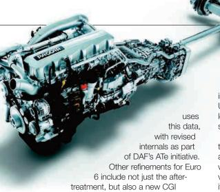
(compacted graphite iron) engine block and highpressure common rail pumps integrated into the block to limit hydraulic losses. Elsewhere, a single auxiliary drive belt and a fan mounted directly to the crankshaft, both save on maintenance costs, and cut weight and fuel usage.
